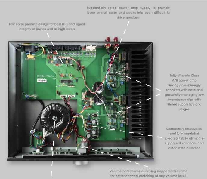
Low noise, generously rated toroidal transformer for clean and ample power reserves
