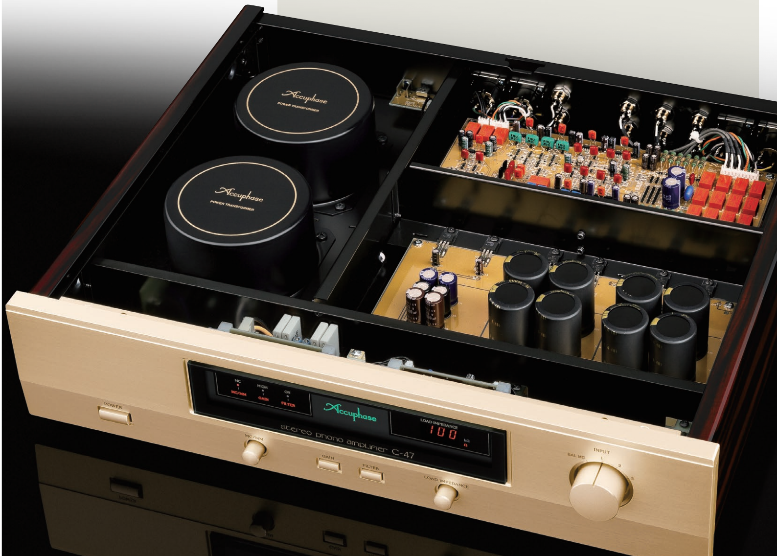
Internal layout realizes full mono construction to prevent mutual interference between channels
